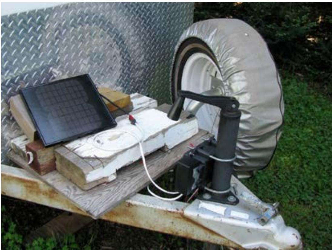
Figure 9: Charger installation showing solar panel.
