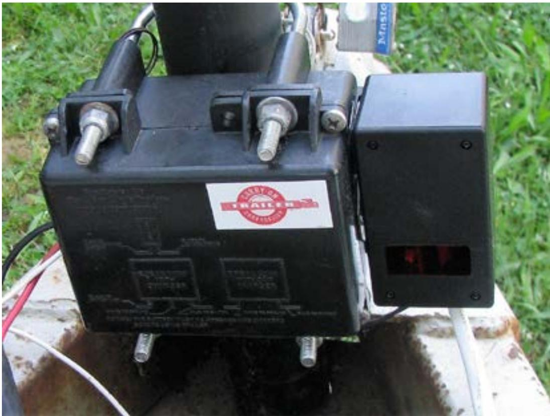
Figure 8. Battery box on left, Solar Float Charger attached on right.
