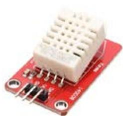
We used an inexpensive sensor to measure temperature and humidity. We displayed it on our Raspberry Pi and also connected it to the Adafruit IO (AIO) cloud so we could see our measurements graphed and displayed on any web browser including a cell phone. We also used AIO to control an LED on our Raspberry Pi from any web browser.
