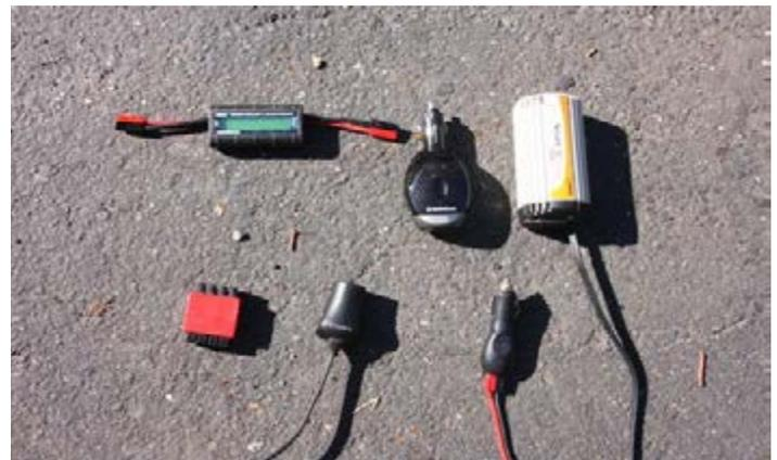
Top: Watt/voltage meter; 2 inverters
