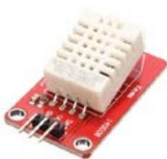
We used an inexpensive sensor to measure temperature and humidity. We displayed it on our Raspberry Pi and also connected it to the Adafruit IO (AIO) cloud so
