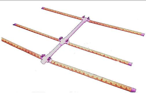
more forward gain, but at the expense of a really good notch in the pattern toward the rear.) It is a design that can be constructed using only simple hand tools (no machine shop needed) and still perform well. It has been duplicated several dozen times by other local hams and has been successfully used as a club construction project.
